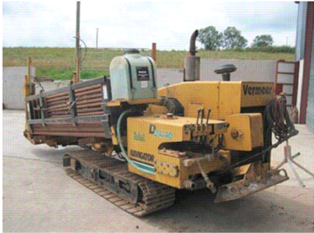
Image 1 : Typical Directional Drilling Rig
